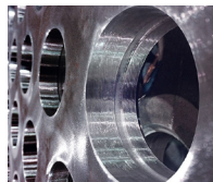
Sure-Lock ring grooves make 40% stronger joints
