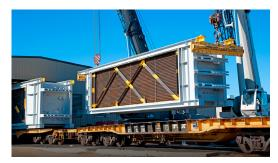
The HORIZON GT-HRSG product solutions are ideally suited for applications use in tandem with gas turbines up to 120+ MW, as well as other process derived heat sources. The modular design combined with custom engineering and shop assembly allows for maximum constructability ease and flexibility on site.
